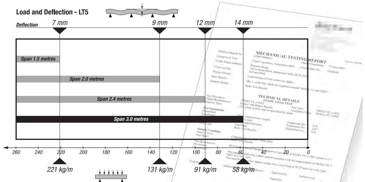
LT5 has been tested in accordance with the NEMA requirements by a NATA certified testing facility. The data displayed is based on physical test results of a 600 wide section and may vary for other widths. The Deflections have been provided as a guide based on continuous spans, and cannot be applied to end spans. Data provided assumes that the installation will be carried out in accordance with NEMA VE2. Non compliance may affect the overall product performance.
