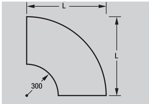
Dimensions do not include integral splice plates. For splice plate, add 100 mm.
