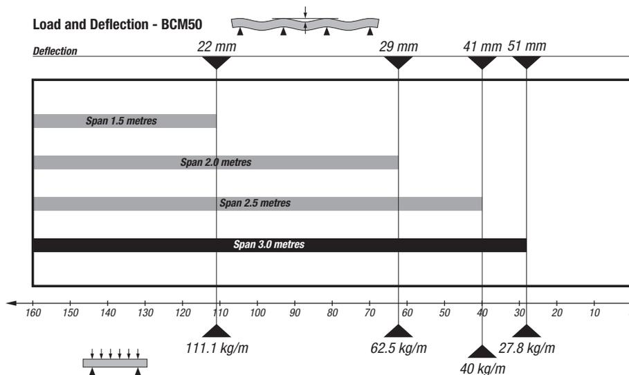
BCM has been tested in accordance with the NEMA requirements. The data displayed is based on physical test results of a 600 wide section and may vary for other widths. The Deflections have been provided as a guide based on continuous spans, and cannot be applied to end spans. Data provided assumes that the installation will be carried out in accordance with NEMA VE2. Non compliance may affect the overall product performance.
