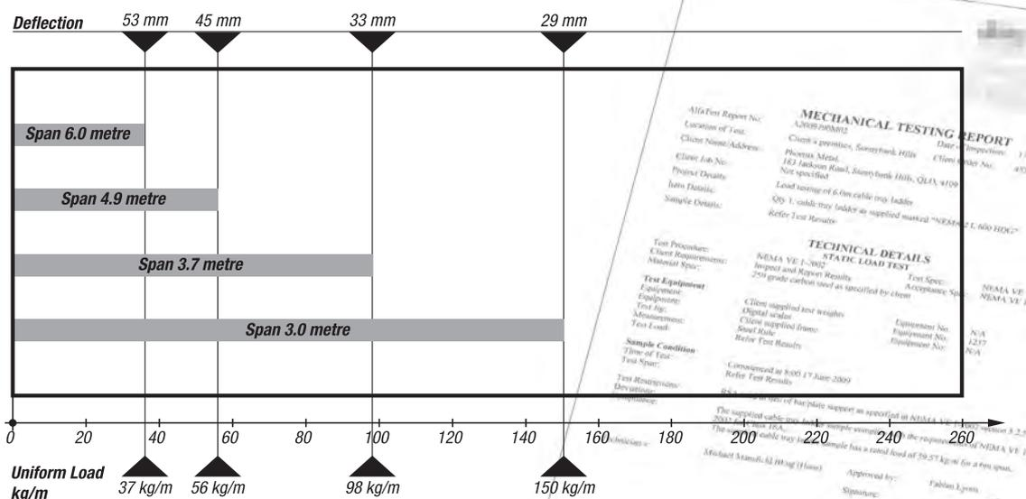
NEMA 1 Cable Ladder has been tested in accordance with the NEMA requirements by a NATA certified testing facility. The data displayed is based on physical test results of a 600 wide section and may vary for other widths. The Deflections have been provided as a guide based on continuous spans, and cannot be applied to end spans. Data provided assumes that the installation will be carried out in accordance with NEMA VE2, non compliance may affect the overall product performance.
