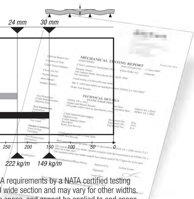
NEMA 4 Cable Ladder has been tested in accordance with the NEMA requirements by a NATA certified testing facility. The data displayed is based on physical test results of a 600 wide section and may vary for other widths. The Deflections have been provided as a guide based on continuous spans, and cannot be applied to end spans. Data provided assumes that the installation will be carried out in accordance with NEMA VE2, non compliance may affect the overall product performance.
