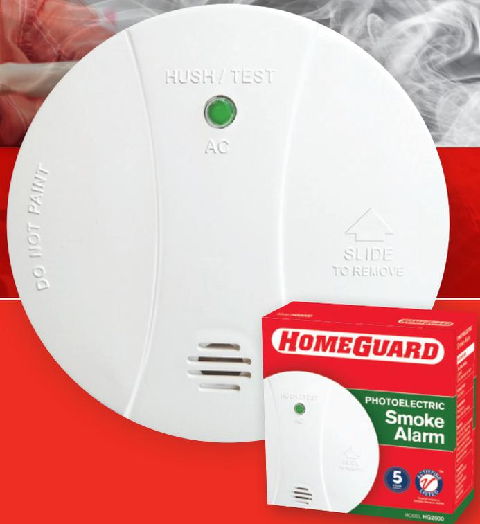
The HOMEGUARD HG2000 is an AC powered, photoelectric smoke alarm that operates on a 240VAC power source with a 9VDC battery backup. This smoke alarm has the ability to function as a stand alone unit or in an interconnected system. This smoke alarm uses photoelectric sensing technology. Photoelectric sensing alarms may detect visible particles (associated with smoldering fires) sooner than ionisation alarms.
