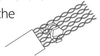
**4)** Untwist and straighten each conductor
