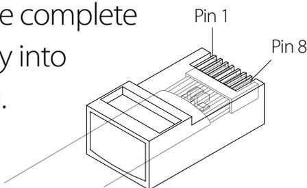
**7)** Finally insert the plug assembly into the crimp tool and crimp the plug to secure the cable.
