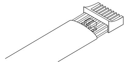
**6)** Insert the complete assembly into the plug.
