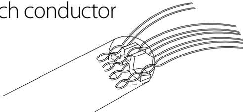
**5)** Trim the conductors (approx 10mm). Insert the conductors into the plastic guide.
